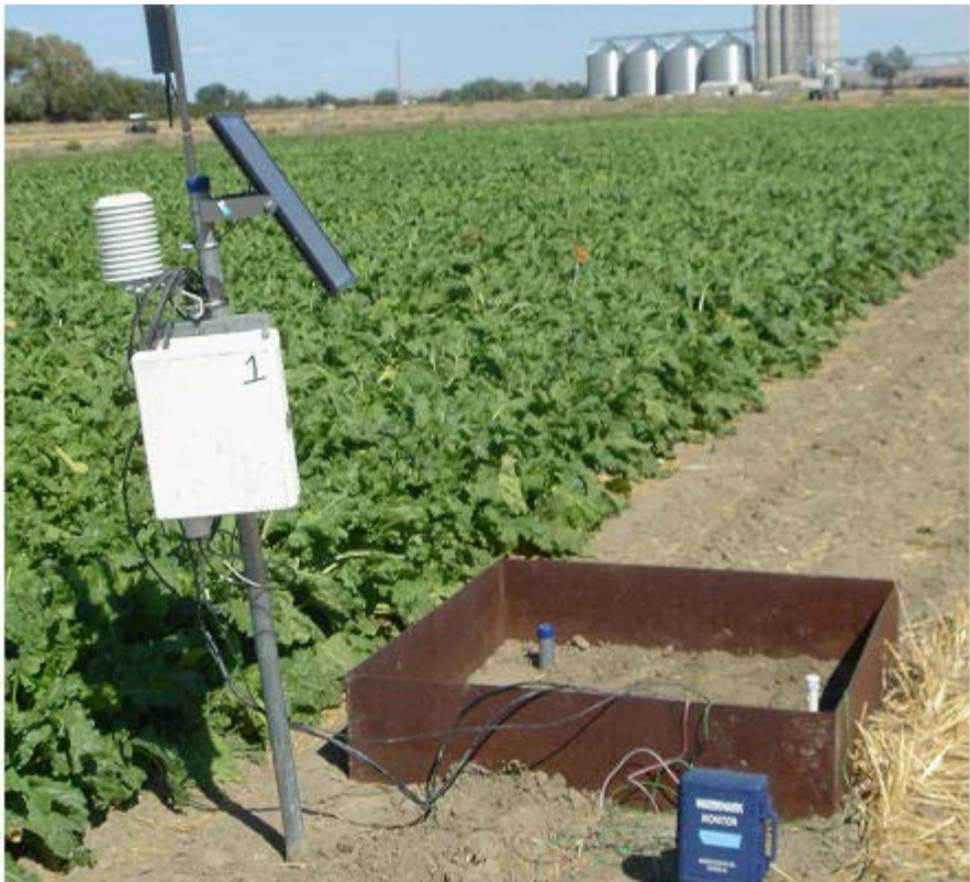
Figure 1. Schematic of the experimental set up. The sensors are installed in the soil inside the metal frame.
