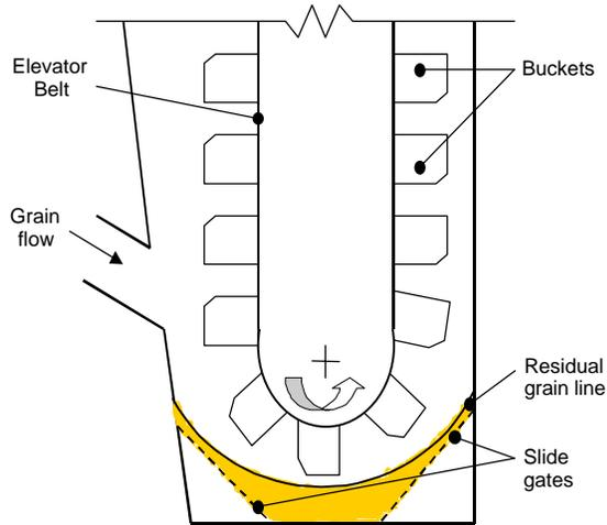
**Figure 5. Schematic diagram of the boot portion of the bucket elevator of the USDA-ARS Grain Marketing and Production Research Center (GMPRC) elevator facility.**
