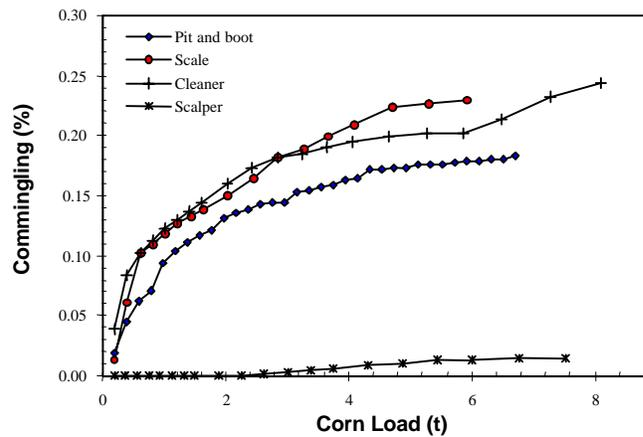
Figure 4. Incremental cumulative commingling for tested handling equipment.
