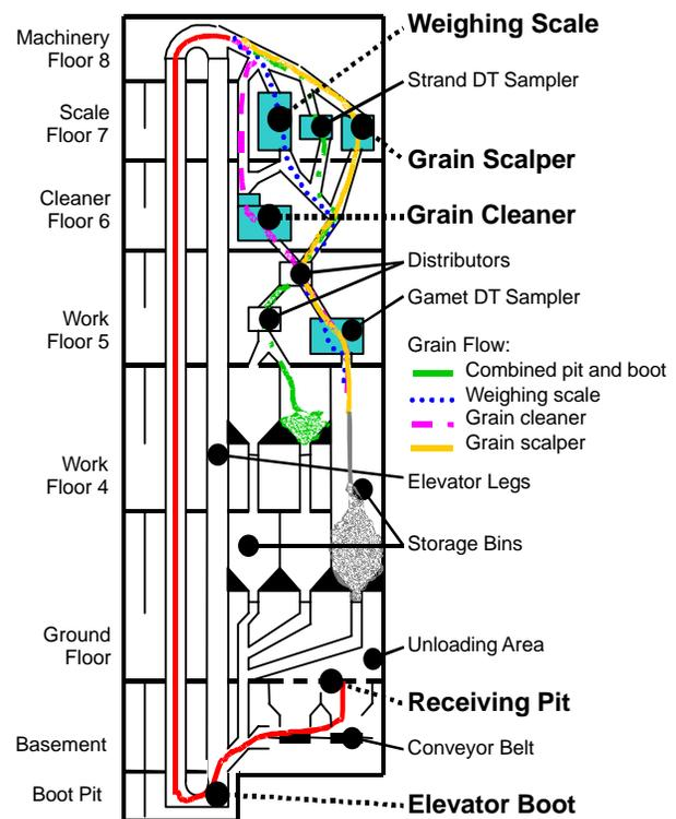
**Figure 1. Grain flowchart and location of handling equipment (names in bold indicate equipment tested in this study).**
