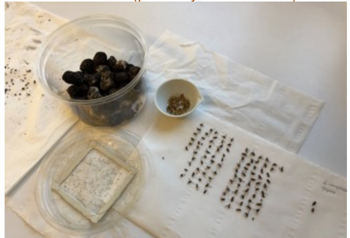
Figure 17. Collection of olive fruit flies after a mesh size test. Flies that managed to escape the container by going through the mesh and flies that remained trapped inside the container were counted, as well as the total number of pupae found in the box. Native parasitoids that were present inside and outside the box were also counted (photo by Gaylord Desurmont).
