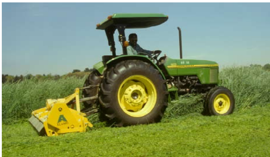
Figure 2. A high-speed flail mower converts the cover crop to a mulch without disturbing the soil.
