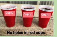
Step 5: Pour ½ cup water in each cup. Wait 1 minute and pour another ½ cup of water in each cup. OBSERVE: Which cup has standing water after a minute? Record answer on data sheet.
