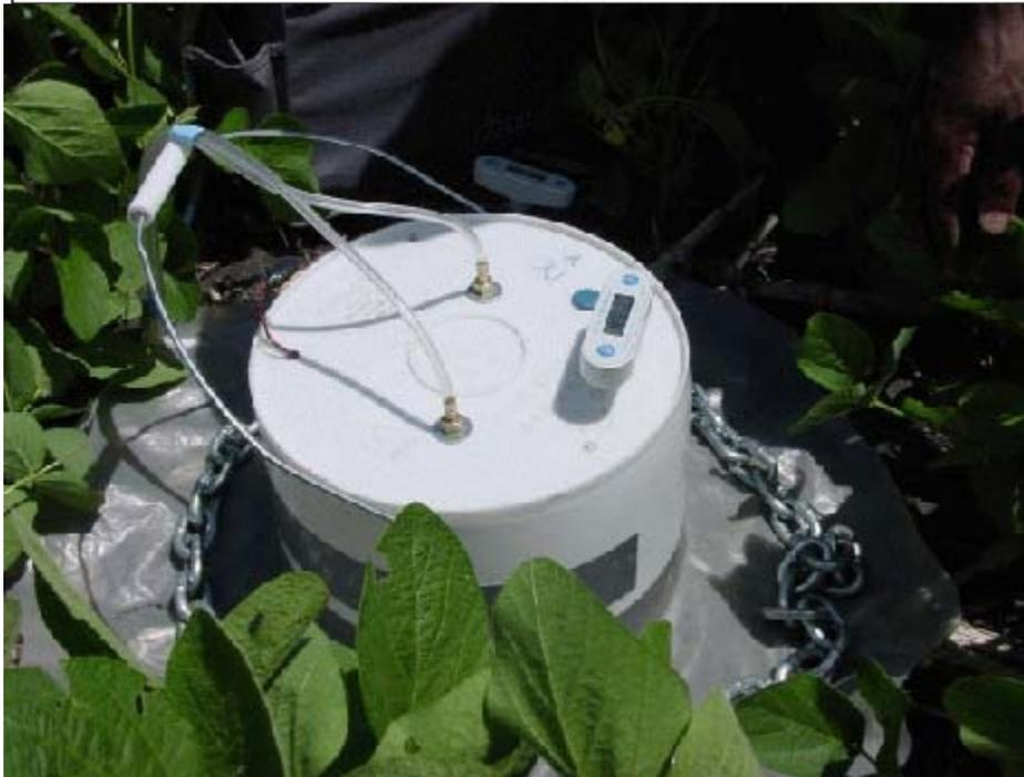
Example of temporary/portable chamber used by Parkin. Chamber has an attached polylethylene skirt held in place on the soil surface with a length of chain. As shown, the chamber is monitoring soil CO<sub>2</sub> flux by recirculating gas through an infrared analyzer. Gas samples can be withdrawn through septum in top of chamber for N<sub>2</sub> and CH<sub>4</sub> analyses.
