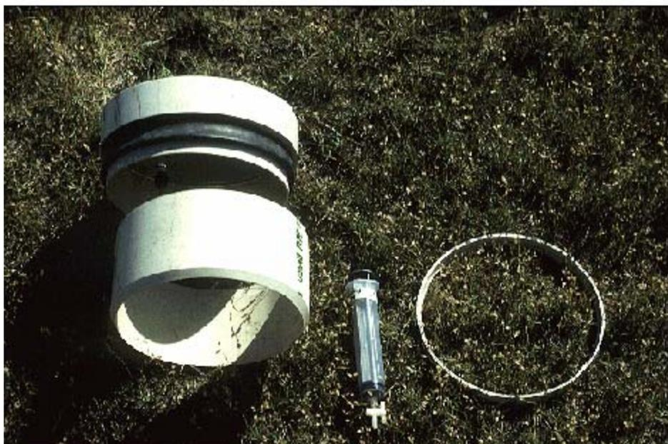
PVC soil anchor and chamber used by Mosier. Rectangular chambers used by Mosier
