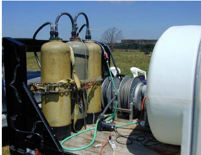
Figure 4. Water filtration tanks on trailer.
