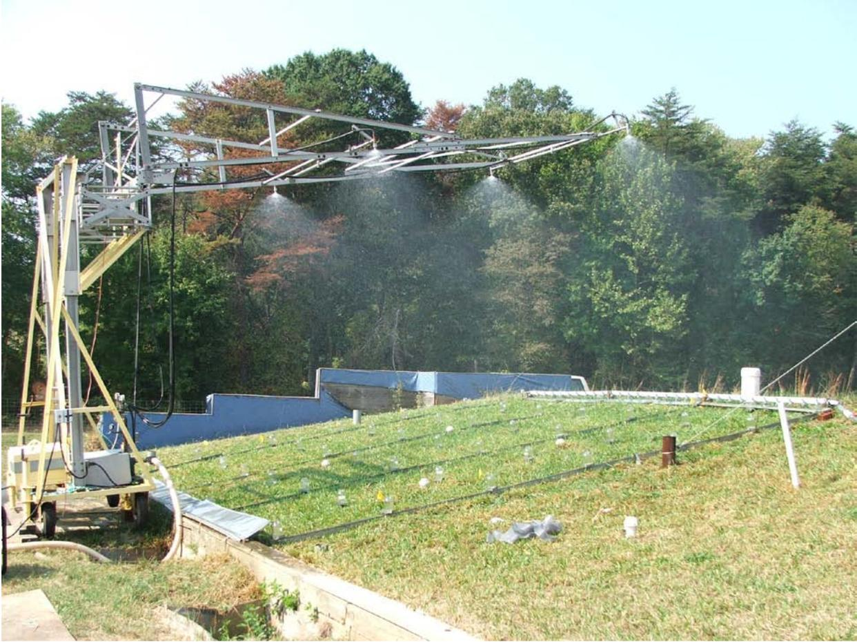
Figure 1. Experimental setup for plot-scale overland flow experiments located at USDA-ARS facility in Beltsville, Maryland.
