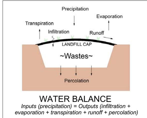
Landfill capping systems reduce the quantity of water moving into and through underlying wastes. Water movement through the organic waste matrix creates leachate, and can result in contamination of ground water and surface water. The effectiveness of a cap design is based on the classical water balance equation based on the principle of conservation of mass:
