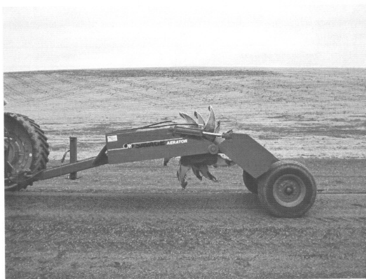
Fig. 2. Rotary subsoiler in transport position.
