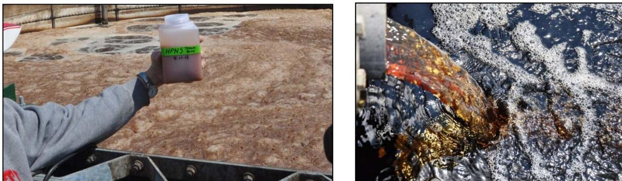
Figure 5. Start-up of the nitrification unit with 1 liter of HPNS (high performance nitrification sludge). Picture at right shows the effluent after N treatment process.
