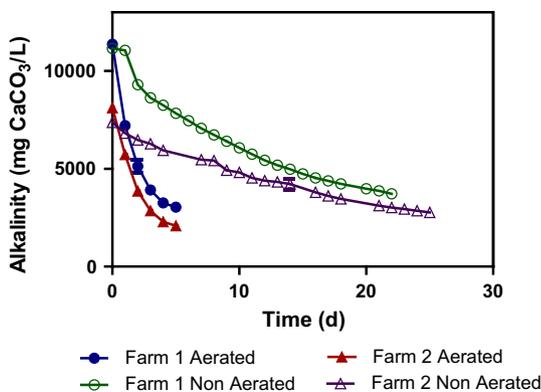
Fig. 5. Effect of aeration on swine wastewater alkalinity during capture of ammonia with gas-permeable membranes. The error bars are standard deviation of duplicate experiments.
