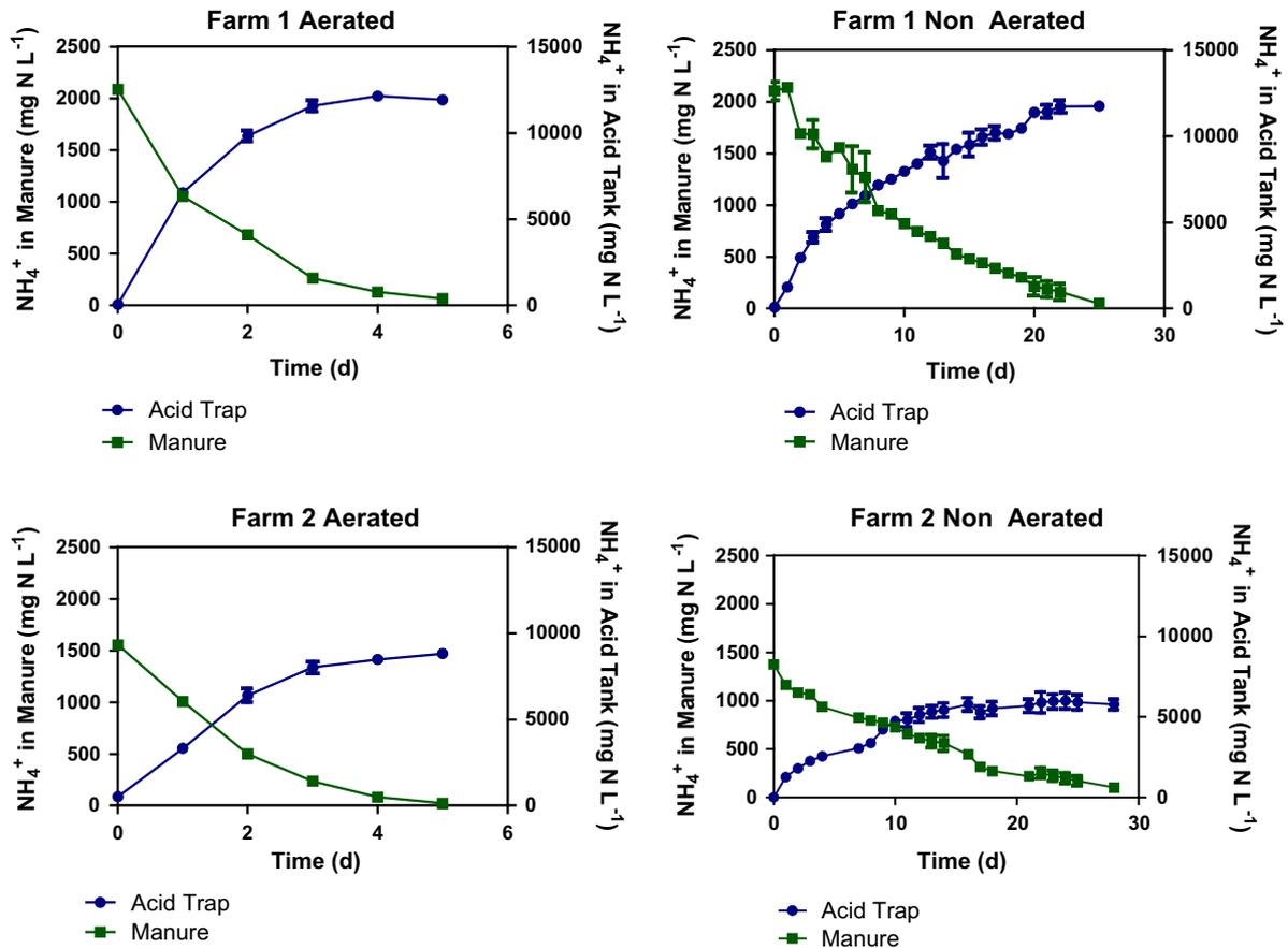
Fig. 3. Effect of aeration on the removal and recovery of  $\text{NH}_4^+$  from digested swine effluent in two farms in North Carolina. The error bars are standard deviation of duplicate experiments.
