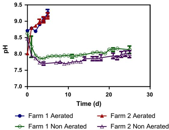
Fig. 4. Effect of aeration on manure pH during recovery of ammonia using gas-permeable membranes. The error bars are standard deviation of duplicate experiments.
