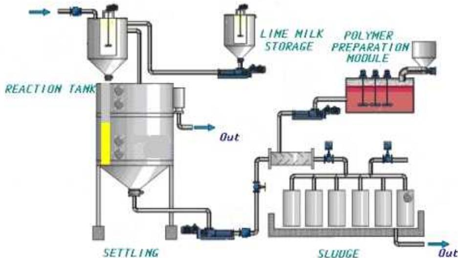
**Figure 6. Schematic diagram of phosphorus separation module constructed in the full-scale manure treatment system demonstration project at Goshen Ridge farm.**
