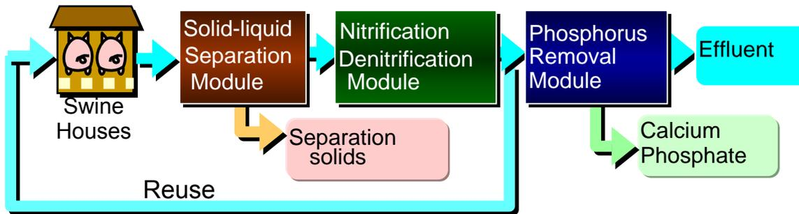
**Figure 2. Diagram of the swine manure treatment system with individual modules implemented at Goshen Ridge farm, North Carolina.**
