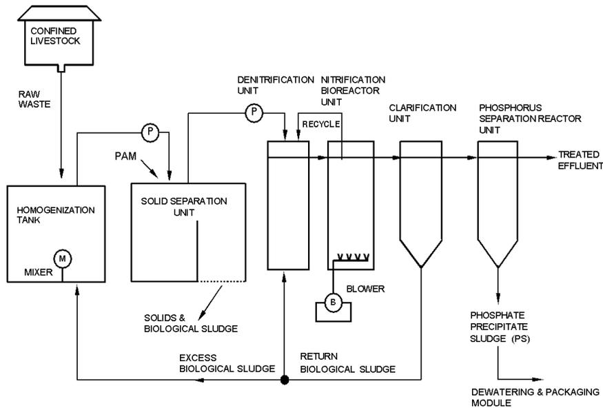
**Figure 1. Schematic of the swine manure treatment system (Vanotti et al., 2005).**
