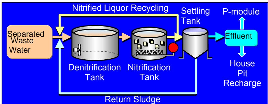
**Figure 5: Diagram of the basic Biogreen process used in the wastewater treatment system for removal of ammonia in swine wastewater after going through solid-liquid separation.**
