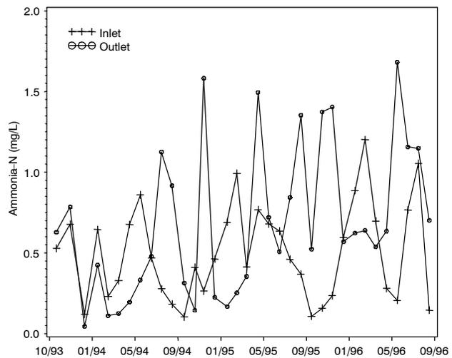
**Figure 5. Mean monthly Ammonia-N inflow and outflow for the in-stream wetland.**
