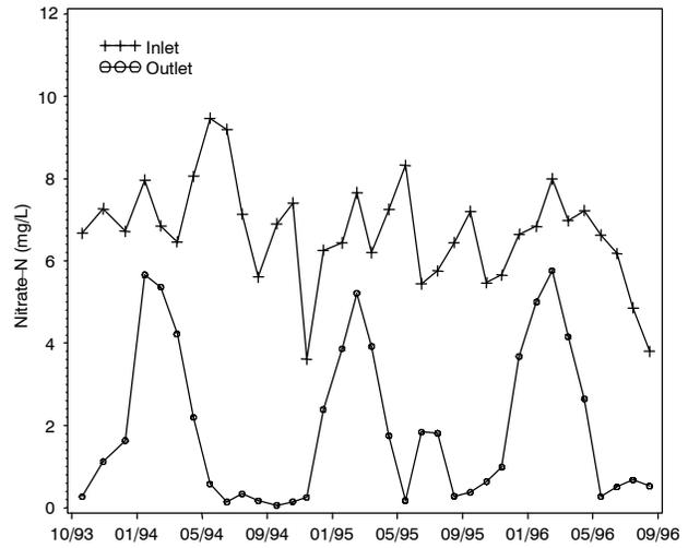
**Figure 4. Mean monthly Nitrate-N inflow and outflow for the in-stream wetland.**
