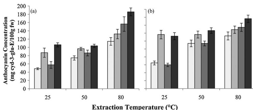
**Fig. 1.** TMA concentration over extraction incubation temperature for (□) 70% ethanol, (■) 70% acidified ethanol, (■) 70% methanol and (■) 70% acidified methanol at (a) 3.3% (w/v) and (b) 17% (w/v) solid loadings.
