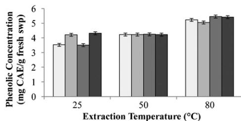
**Fig. 2.** Phenolic concentration over extraction temperature for (□) 70% ethanol, (■) 70% acidified ethanol, (■) 70% methanol and (■) 70% acidified methanol, across solid loading.
