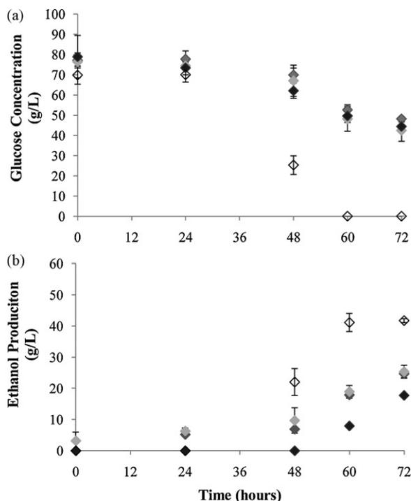
Fig. 6. (a) Glucose concentration and (b) ethanol production within the 5.0 AGU/g dry ISP enzyme loading over fermentation incubation time for extraction conditions of (◆) acidified ethanol at 50 °C, (◆) acidified ethanol at 80 °C, (◆) acidified methanol at 80 °C, (◇) no extraction fermentation control.
