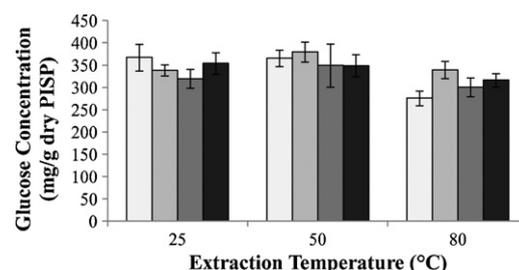
**Fig. 4.** Glucose concentration after hydrolysis over extraction temperature for (□) 70% ethanol, (■) 70% acidified ethanol, (■) 70% methanol and (■) 70% acidified methanol, across solid loading.
