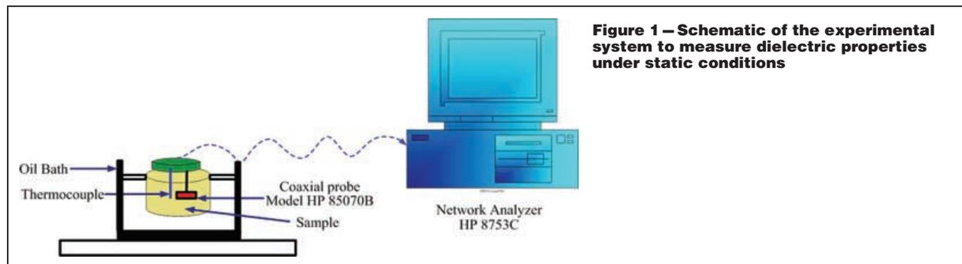
**Figure 1 – Schematic of the experimental system to measure dielectric properties under static conditions**
