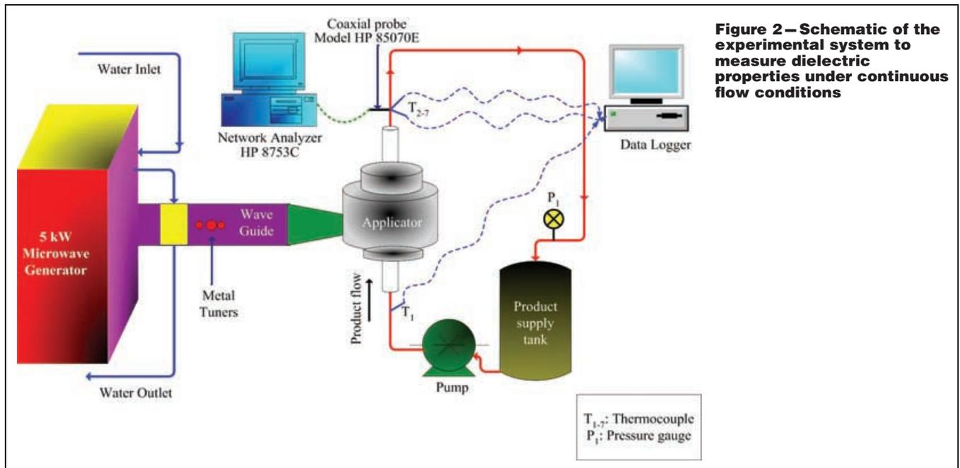
**Figure 2 – Schematic of the experimental system to measure dielectric properties under continuous flow conditions**
