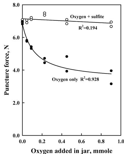
**Figure 5.** Effect of the addition of oxygen only (●) or oxygen + 2.3 mM sulfite (○) on the firmness stored red bell peppers. Jars of peppers were filled in an anaerobic hood, oxygen and sulfite were injected as shown, and the peppers were stored for 3 weeks in 150 mM acetic acid and 12 mM sodium benzoate, pH 3.5.
