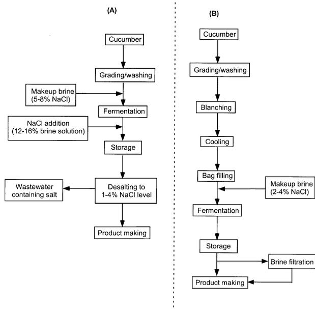
**Figure 1.** Flow chart of the traditional (A) and controlled (B) fermentation processes (Fleming et al., 2002).
