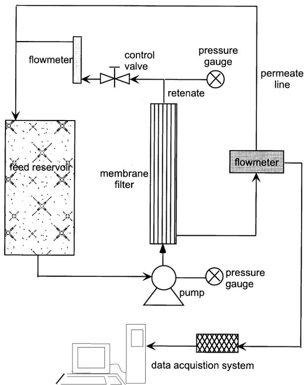
Figure 2. Schematic diagram of crossflow filtration process.
