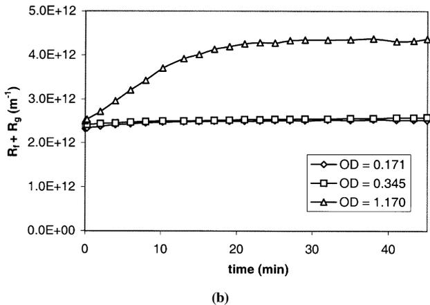
Figure 5. Flux decline curves and cake resistance at different flow rates for brine (OD = 0.171) filtered through 0.2- $\mu$ m membrane. Transmembrane pressure was 103 kPa.
