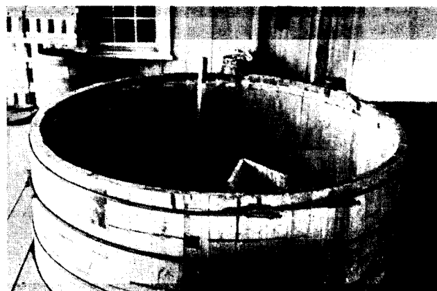
Fig. 2. Pasteurizing tank showing "V" circulation baffle in front.
