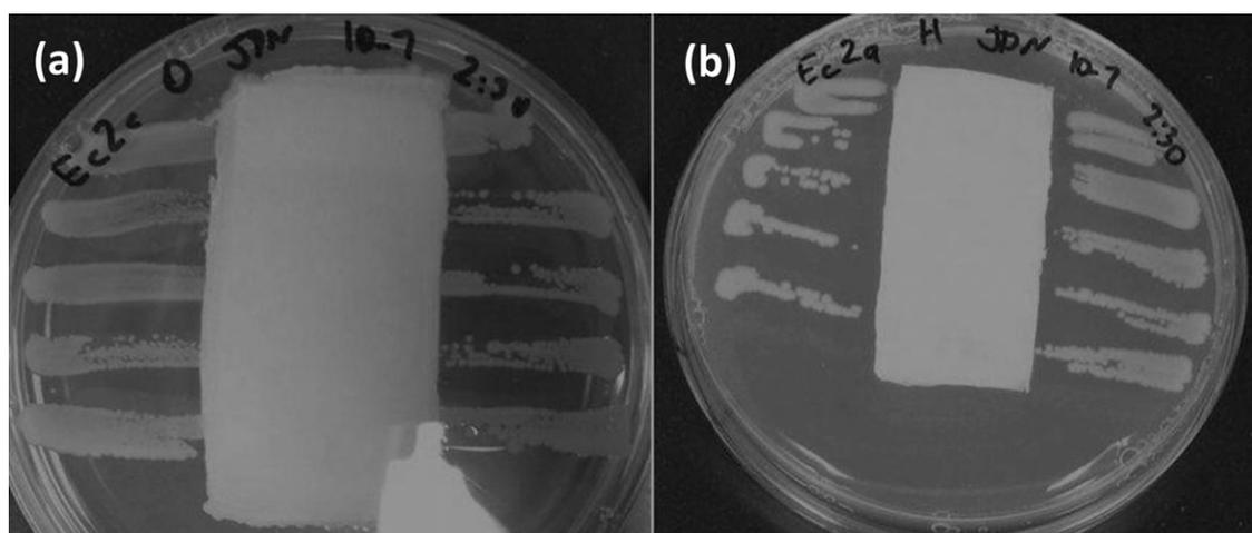
**Figure 9.** AATCC 147 Gram-negative (*E. coli*) testing plates of (a) Nylon/cotton fabric; (b) Ag/PAN nanofiber-deposited Nylon/cotton fabric (Ag precursor concentration: 1.25 wt %; nanofiber area density: 1.87 g/m<sup>2</sup>).
