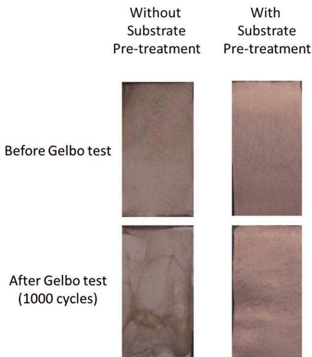
**Figure 12.** Gelbo Flex test results of Ag/PAN nanofiber-deposited Nylon/cotton fabrics. Nanofiber area density: 1.87 g/m<sup>2</sup>.
