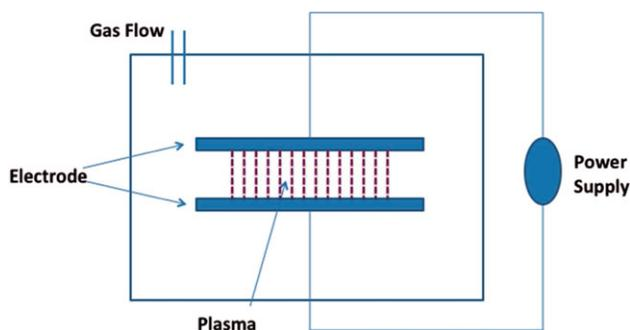
**Figure 1.** Schematic of the atmospheric plasma device NCAPS. [Color figure can be viewed in the online issue, which is available at [wileyonlinelibrary.com](http://wileyonlinelibrary.com).]
