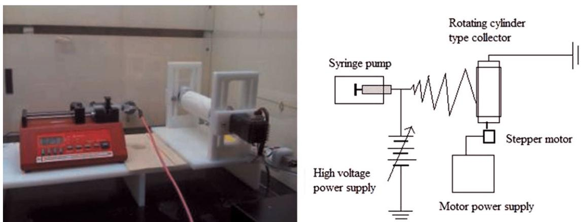
**Figure 2.** Photograph and schematic diagram of the electrospinning setup. [Color figure can be viewed in the online issue, which is available at [wileyonlinelibrary.com](http://wileyonlinelibrary.com).]
