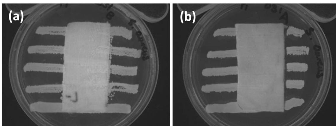
**Figure 10.** AATCC 147 Gram-positive (*S. aureus*) testing plates of (a) Nylon/cotton fabric; (b) Ag/PAN nanofiber-deposited Nylon/cotton fabric (Ag precursor concentration: 1.25 wt %; nanofiber area density: 1.87 g/m<sup>2</sup>).
