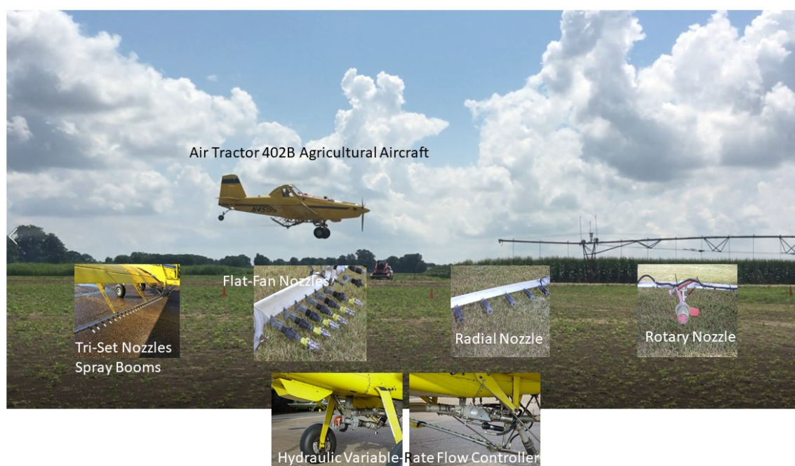
Fig. 2 Air Tractor 402B with spray booms and flow control system for different nozzles used for aerial application research in Stoneville, Mississippi.
