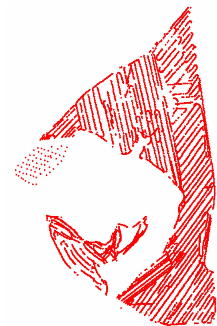
Figure 3. Deep Hollow Watershed topographic survey points
