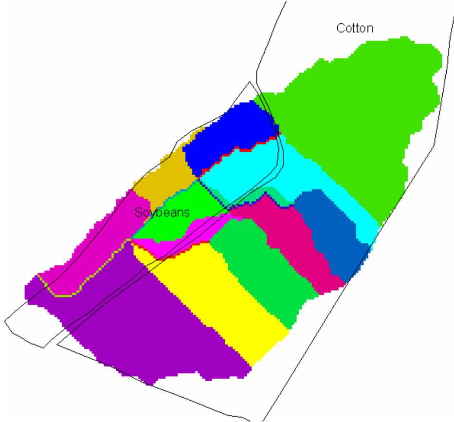
Figure 16. Overlay of land use information on the delineated watershed and subwatersheds for monitoring flume UL2
