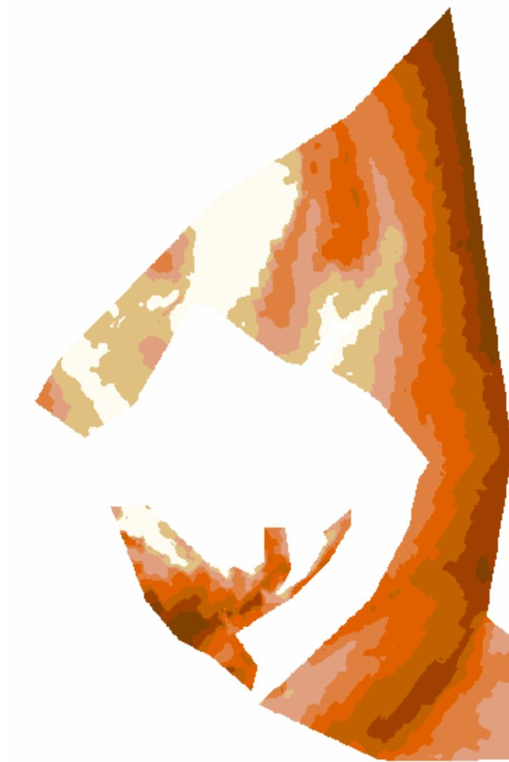
Figure 9. Generated DEM based on the topographic survey
