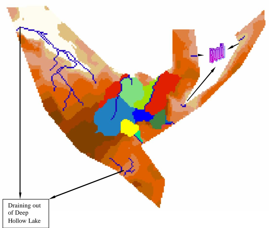
Figure 12. Drainage areas and their boundaries for the small area of Deep Hollow Lake
