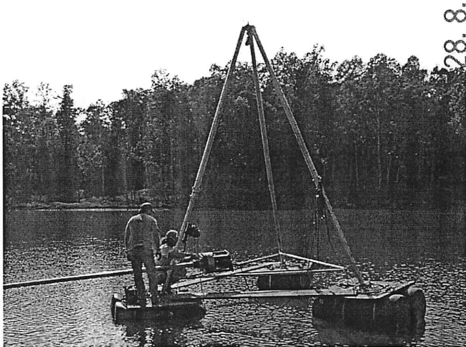
Figure 7. Photograph of floating vibracore system showing the tripod and portable rafts. A core pipe is being connected to the vibracore head (September 2000).
