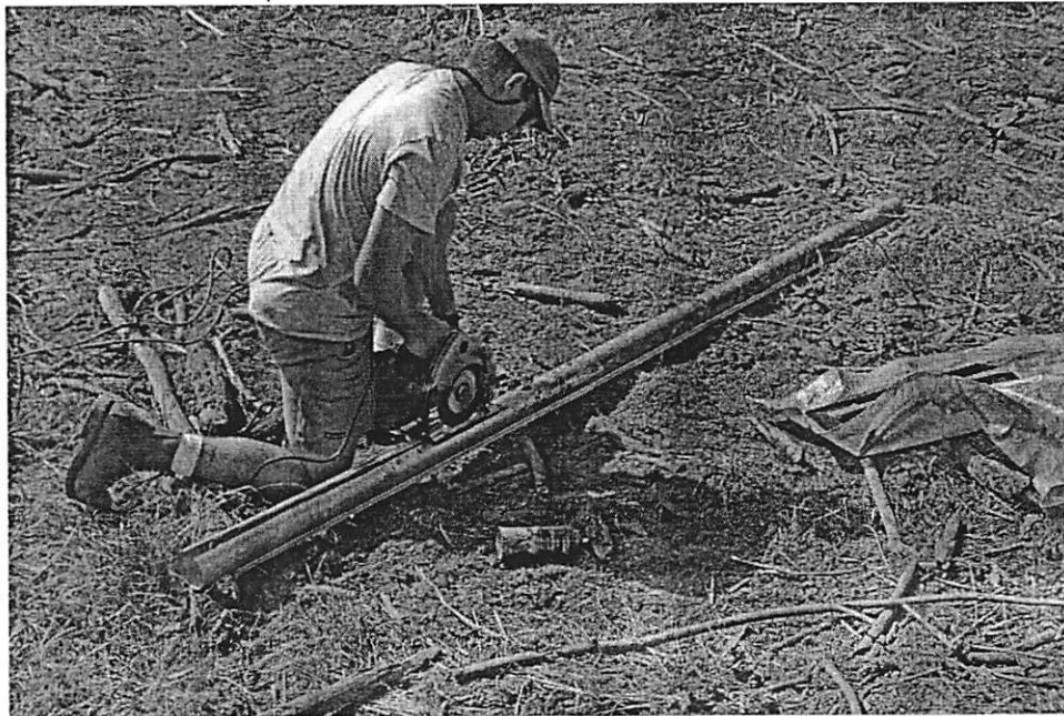
Figure 10. Photograph of extracted core being cut open on-site (photograph taken in Oklahoma, June 2000).
