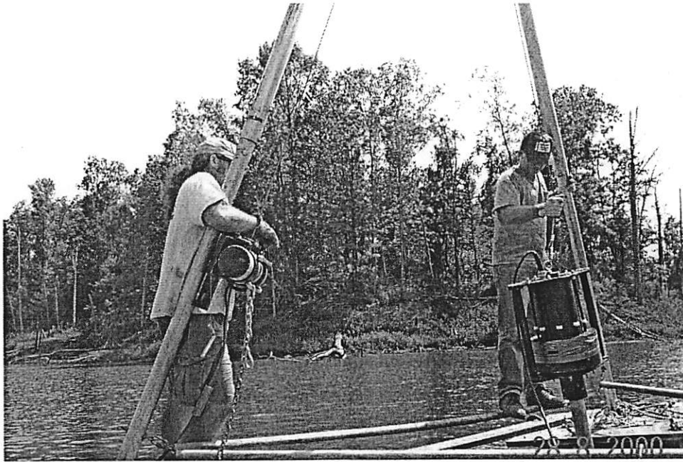
Figure 9. Photograph of vibracore system showing the tripod, vibracore head, and winch and cable assembly (September 2000).
