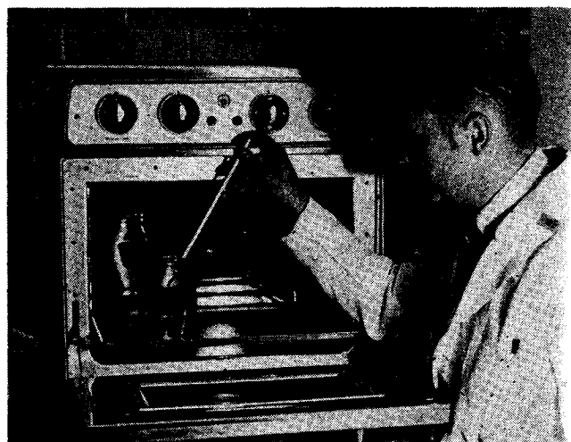
Fig. 2. Determining the temperature of honey liquefied in a microwave oven.
