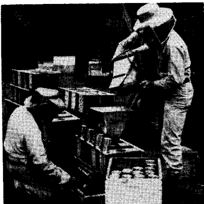
Packages are crated before filling and weighed individually when filled from the shaker box. (Texas)
