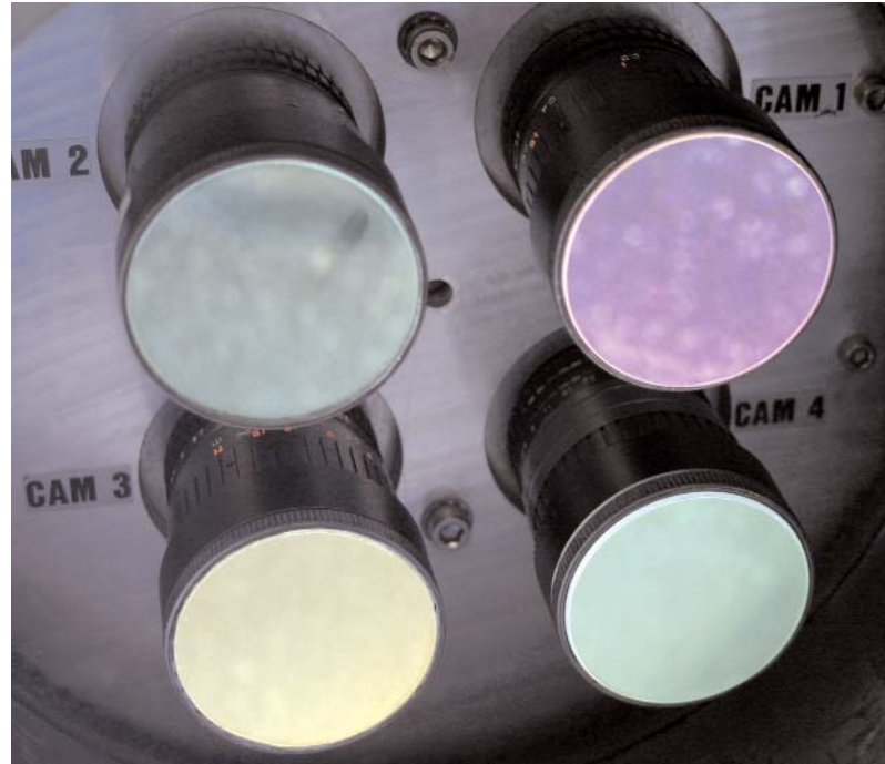
Extending through the belly of the aircraft, each of the lenses pictured above captures a separate spectral band including red, blue, green, and near-infrared (NIR)
