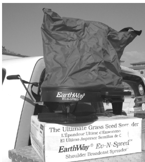
Figure 2. Model 2700-A Earthway EV-N-SPRED Broadcast Seeder/Spreader used in the metaflumizone EUP broadcast RIFA control study. Miller Co. AR. 2006.
