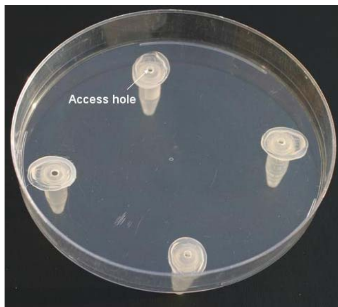
Figure 1. Bioassay apparatus for evaluating fire ant repellents.
