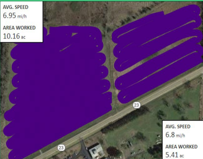
Field path with sub-meter tractor guidance technology (left) and without tractor guidance (right) on adjacent hay fields at the USDA-ARS Small Farms Research Center in Booneville, AR, 2018. Both fields used the same fertilizer spreader, tractor, and tractor operator.
