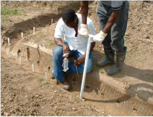
Figure 3. Inserting plastic rulers for soil erosion study in freshly constructed quarter-drain using a custom made knife to cut 15-cm deep soil opening, and a pushing tool to place each ruler at the exact same depth.
