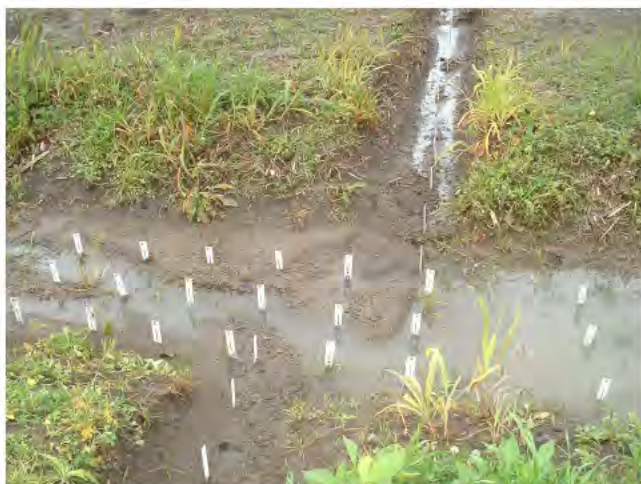
Figure 6. Sediment deposition at the cross-section between two quarter-drains and the main field ditch after the third rainfall event (90 mm depth).
