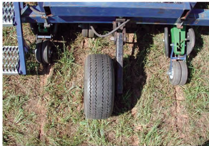
Fig. 1. Bermudagrass pasture after subsurface band application of poultry litter using a four-row prototype banding implement.
