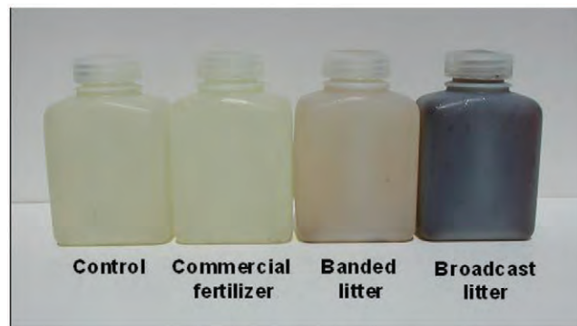
Fig. 4. Cumulative treatment impacts on clarity of runoff water from the rainfall simulation event.
