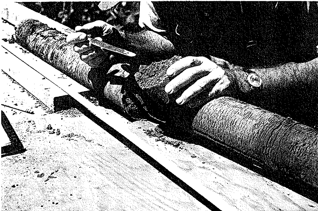
Fig. 2. A technician is counting the number of roots that project from the 2 broken surfaces of a soil core in the core-break technique.
