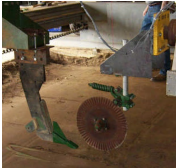
Figure 2. Subsoiler system mounted on the three-dimensional dynamometer in the NSDL soil bins.
