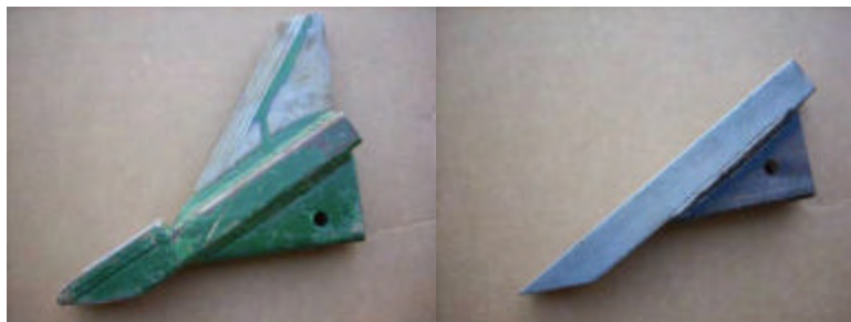
Figure 1. Points used in the soil bin experiment. On the left is the splitter point (SP) and on the right is the standard ripper point (P).
