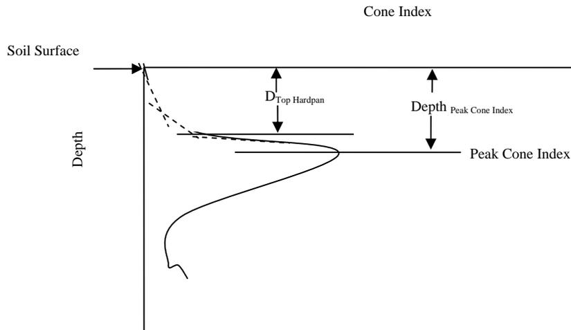
Figure 1. Cone index vs. depth to determine the depth to the peak cone index ( $D_{\text{Top Hardpan}}$ ) and the depth to the top of the hardpan layer ( $D_{\text{Hardpan}}$ ). The instantaneous slope values are shown as straight dashed lines that are tangent to the curve.
