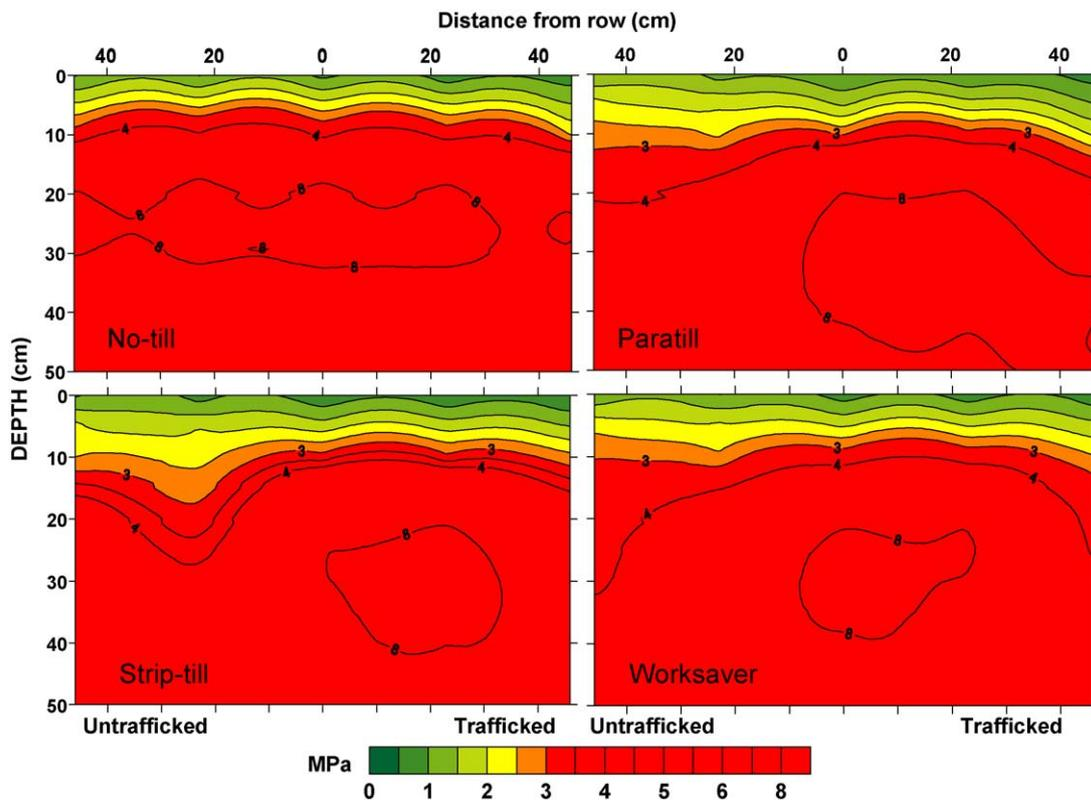
Fig. 3. Spring 2006 soil strength of a Dothan sandy loam in southeastern AL before tillage for cotton planting. The four tillage treatments averaged across cover crop treatments as influenced by row position and depth. Isolines created by Kriging interpolation.
