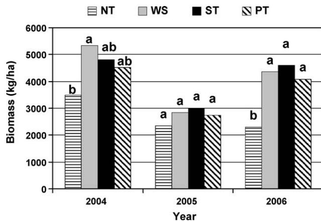
Fig. 1. Annual winter rye cover crop biomass production as affected by in-row subsoiling (NT—no-till; WS—worksaver; ST—strip-till; PT—paratill). Different lower case letters indicate statistical significance  $LSD_{0.1}$  within year.
