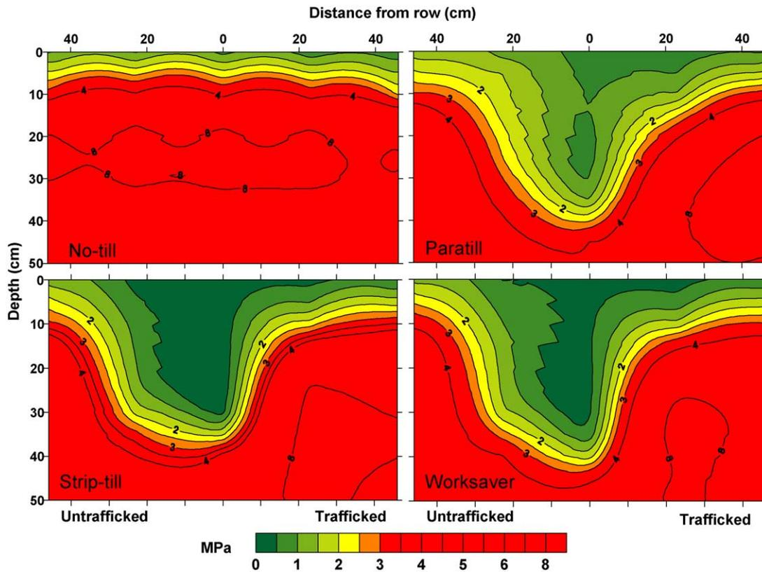
Fig. 4. Spring 2006 soil strength of a Dothan sandy loam in southeastern AL after tillage for cotton planting. The four tillage treatments averaged across cover crop treatments as influenced by row position and depth. Isolines created by Kriging interpolation.
