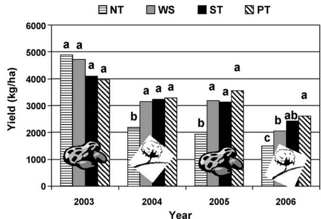
Fig. 7. Peanuts and cotton yields as affected by in-row subsoiling. Letters indicate NT—no-till; WS—worksaver; ST—strip-till; PT—paratill. Different lower case letters indicate statistical significance LSD<sub>0.1</sub>.
