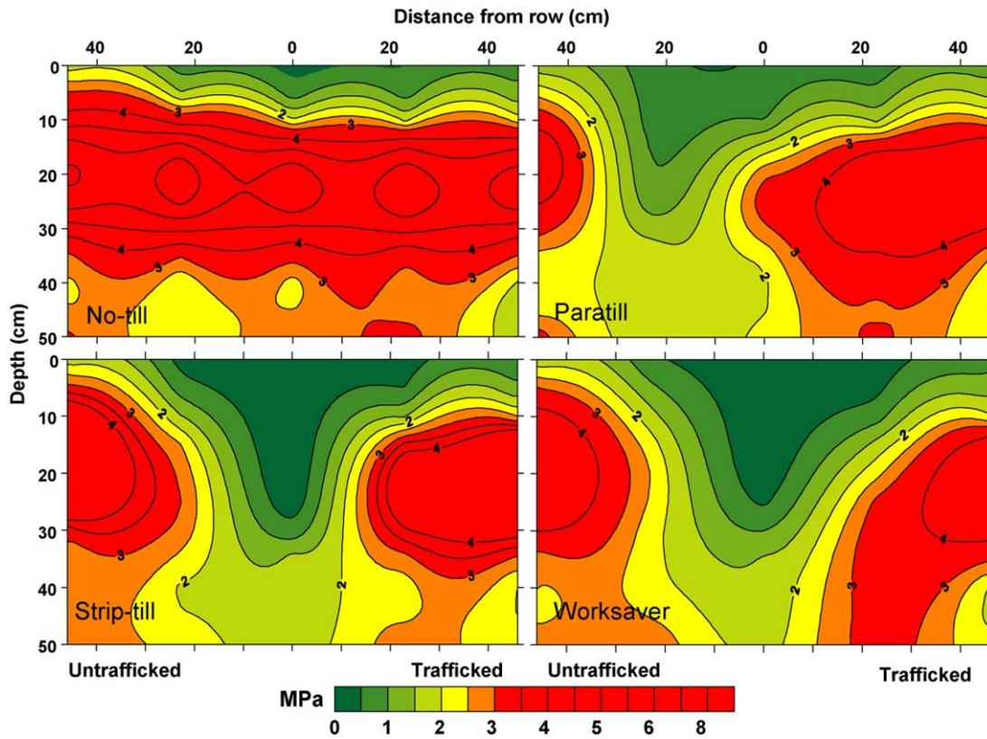
Fig. 2. Spring 2005 soil strength of a Dothan sandy loam in southeastern AL after planting the peanut crop. The four tillage treatments averaged across cover crop treatments as influenced by row position and depth. Isolines created by Kriging interpolation.
