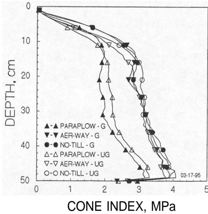
**Figure 2.** Cone index profiles one year after tillage practices were conducted. The 'G' and 'UG' designations indicate grazed and ungrazed, respectively
