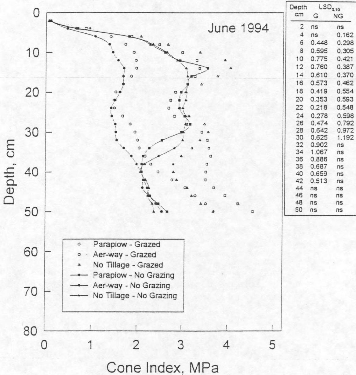
Figure 1. Cone index (June 1994) at 25 soil depths as influenced by renovation tillage treatments in a tall fescue-bermudagrass pasture, Crossville AL. G = grazed; NG = not grazed; ns = not significant ( $P \leq 0.10$ ).
