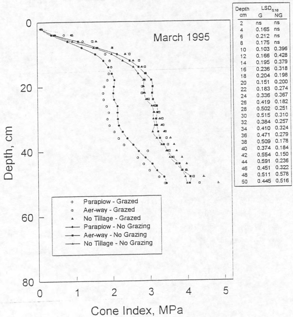
Figure 2. Cone index (March 1995) at 25 soil depths as influenced by renovation tillage treatments in grazed and ungrazed tall fescue-bermudagrass pasture, Crossville AL. G = grazed; NG = not grazed; ns = not significant ( $P \leq 0.10$ ).
