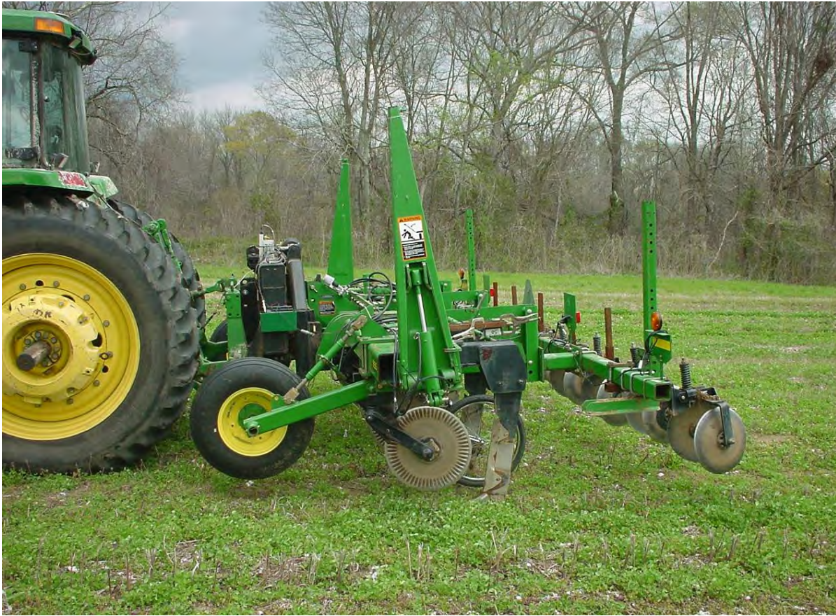
Figure 4. John Deere 955 used for subsoiling treatments.
