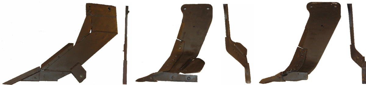
Figure 1. Side and front views of KMC subsoiler (left), Paratill™ (center), and Terratill™ (right) used in the experiment.
