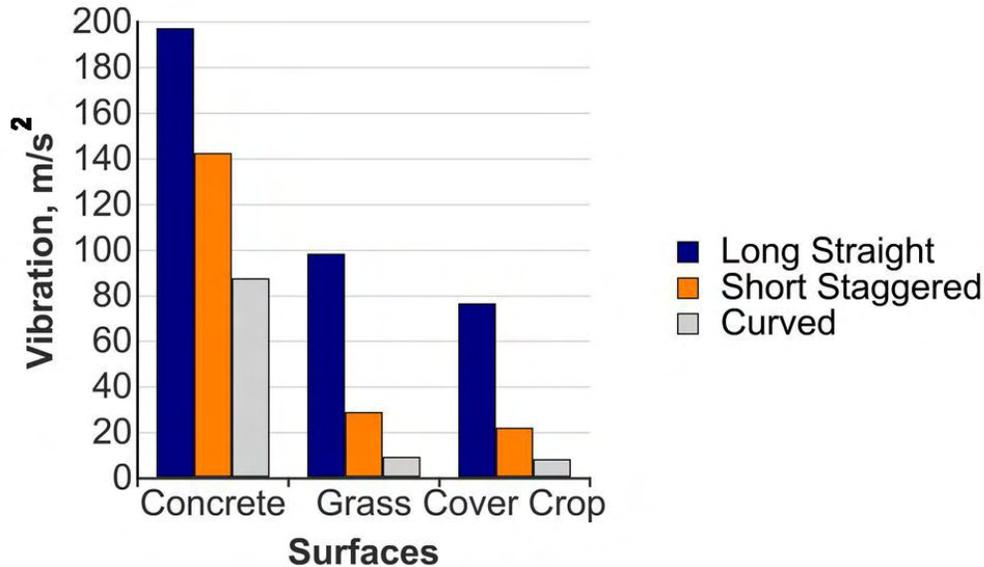
Figure 6. Vibration data obtained with the experimental roller for Experiment 3.  $LSD_{0.1}$  between surfaces within treatments =  $6.9 \text{ m/s}^2$ ;  $LSD_{0.1}$  between treatments within surfaces =  $5.8 \text{ m/s}^2$ .
