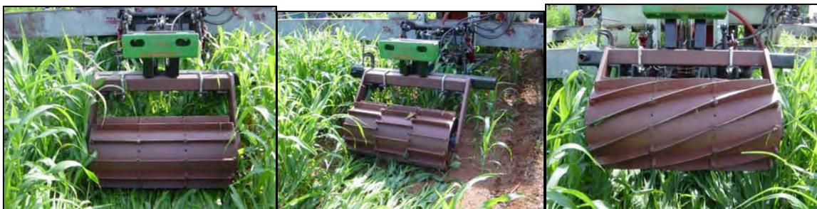
Figure 2. Small roller used for Experiments 2 and 3. On the left is the long-straight blade system, in the center is the short-staggered straight blade system, and to the right is the curved blade system.
