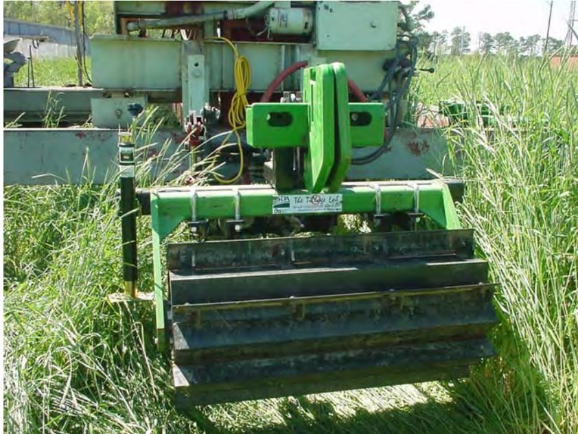
Figure 1. Small section of a cover crop roller used for Experiment 1 in the soil bins of the NSDL. A weight bracket and two weights are shown mounted on the roller. Also, note the blades mounted on the roller as well as the angle iron mounted between the blades.
