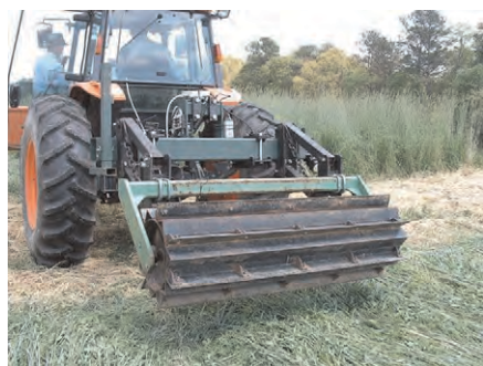
Fig. 1. Rolling cover crops using a 2.8-m straight bar roller/crimper with 6-mm thick blunt crimping bars.
