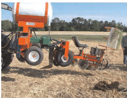
Fig. 3. Side view of the modified RJ transplanter showing the subframe with the subsoiler shank and two ground-driven wheels to power the moving components.
