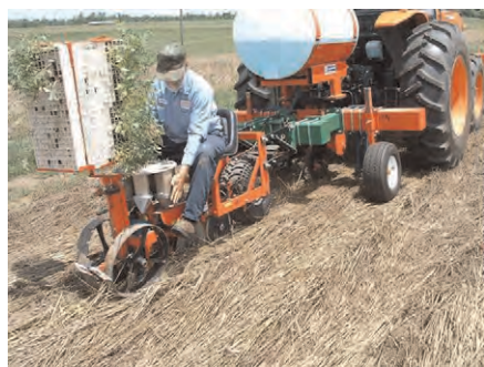
Fig. 2. Planting tomato seedlings into rolled rye residue cover using a modified RJ no-till transplanter from RJ Equipment Company, Blenheim, Ontario, Canada.
