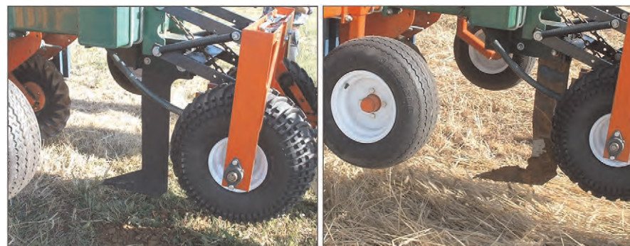
Fig. 4. Two different shank subsoilers used. On the left, the slim 13 mm thick; and on the right, wide-shank 20-mm thick mounted on the transplanter. Note that the overall shapes of the two shanks were similar.
