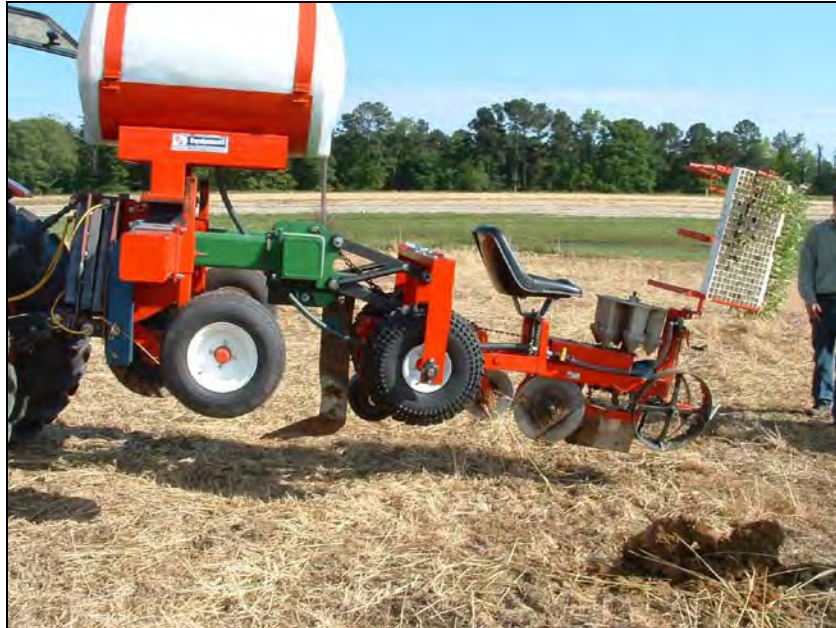
Figure 3. Side view of the RJ transplanter showing the sub-frame with the subsoiler shank and two powered wheels
