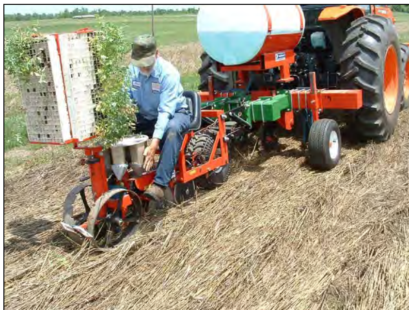
Figure 2. Planting tomato seedlings into rolled rye residue cover using a modified RJ No-till transplanter from RJ Equipment Company, Blenheim, Ontario
