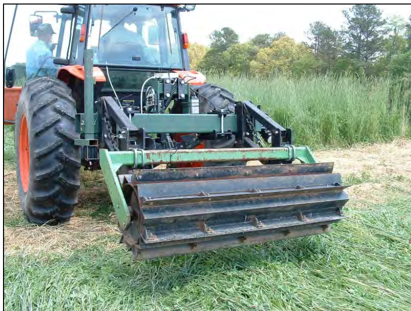
Figure 1. Rolling cover crops using a 8 ft straight bar roller/crimper with ¼ inch thick crimping bars
