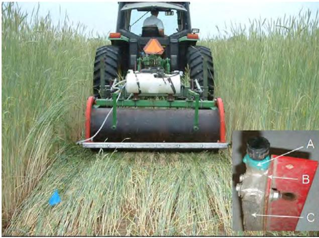
**Figure 2.** Glyphosate discharge assembly from felt strip mounted to the crimping bar: (A) sealed soak-type garden hose; (B) crimping bar; (C) felt strip material.
