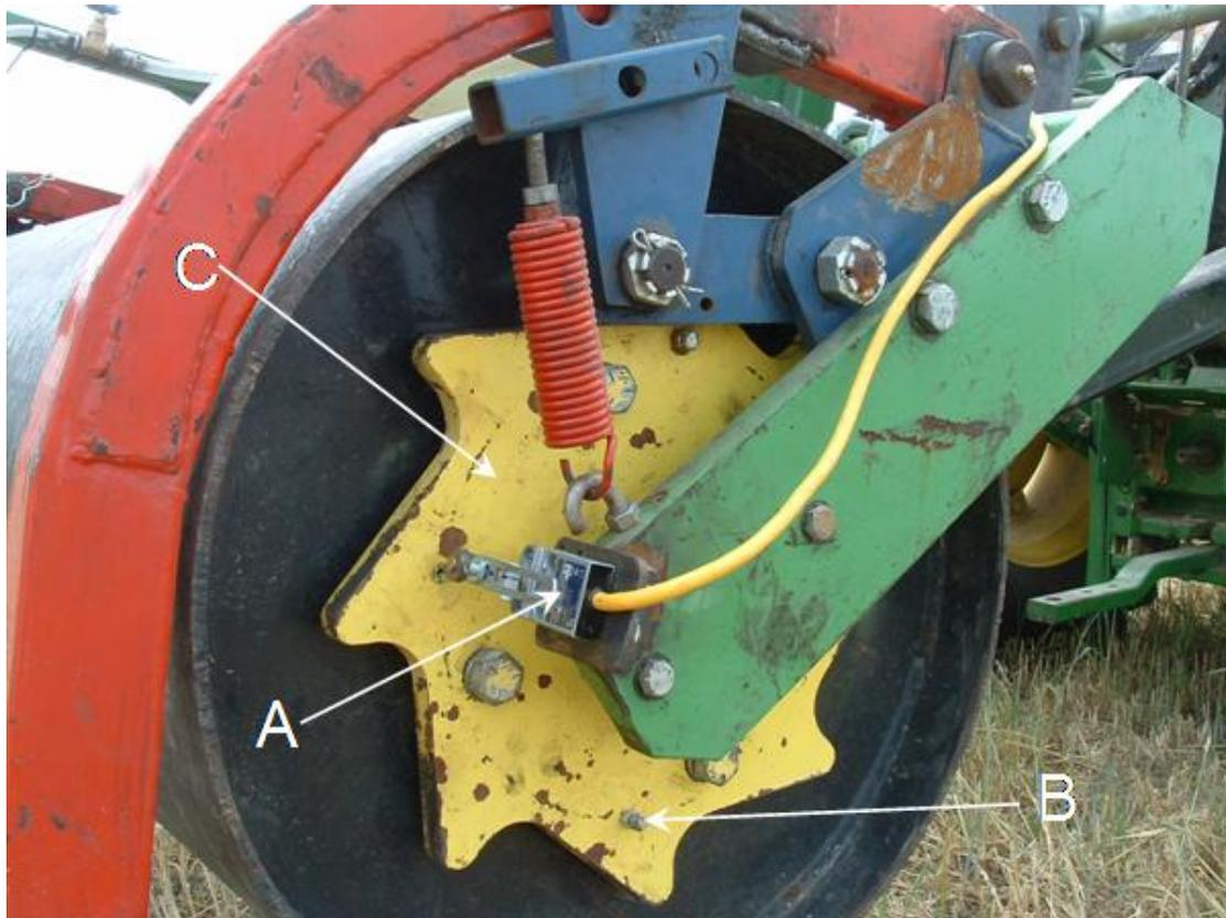
Figure 4. Side view of the smooth roller with crimping bar. A. Micro-switch; B. Engagement bolt with the switch's arm; C. Eight-cam crimping bar control mechanism with clockwise rotation.
