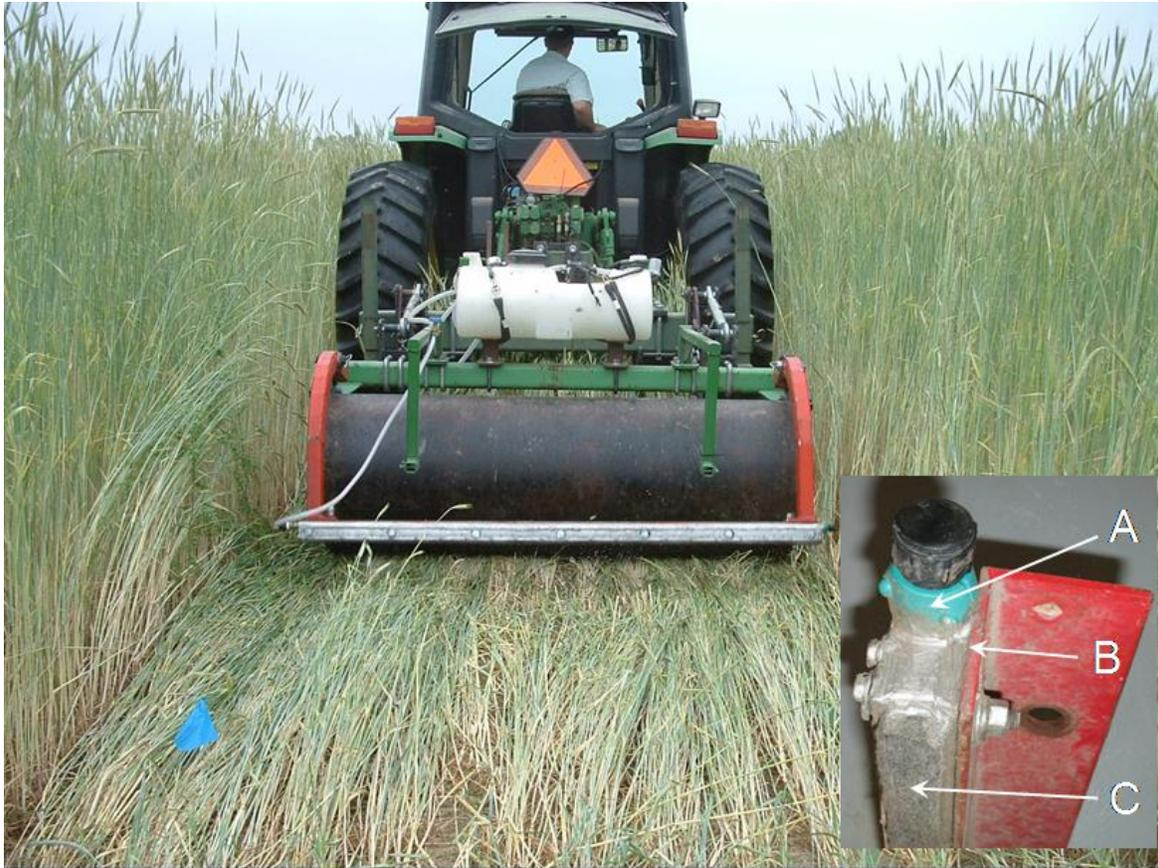
Figure 2. Roundup discharge assembly from felt strip mounted to the crimping bar: A. sealed soak-type garden hose; B. crimping bar; C. Felt strip material.
