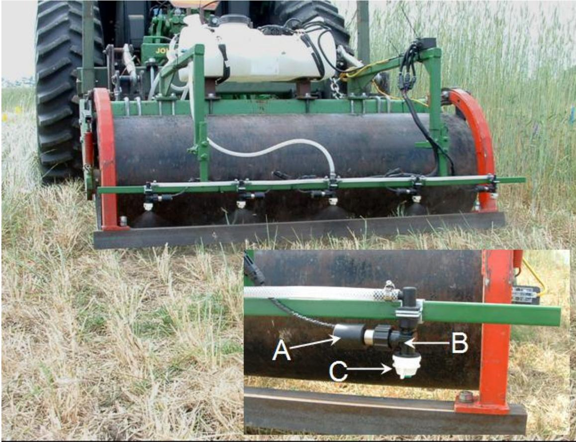
Figure 3. Back view of the smooth roller with crimping bar and the attached high speed solenoid valve: A. Solenoid valve, B. Nozzle body, C. Nozzle.
