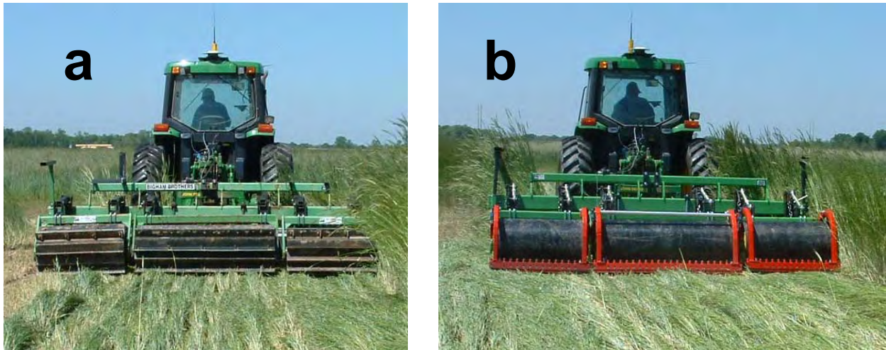
Figure 1. Three-section roller types: (a) Straight bar roller, and (b) Smooth roller/crimper.
