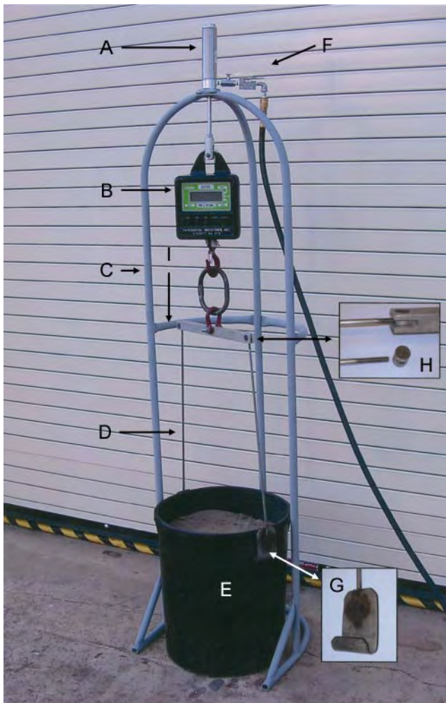
Fig. 1. Photograph of weighing system positioned around a container to be weighed: (A) pneumatic cylinder, (B) hanging scale, (C) support frame, (D) lifting arm apparatus, (E) 45-L container filled with soil, (F) trigger mechanism for activating the pneumatic cylinder connected to compressed air source, (G) bent plate to catch container handle during lifting, (H) close-up view of one end of the top horizontal bar, and (I) middle “U”-shaped support tubing attached to upright frame.
