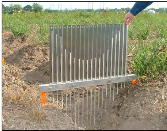
Figure 2. Portable device to measure soil erosion/deposition in quarter-drain.
