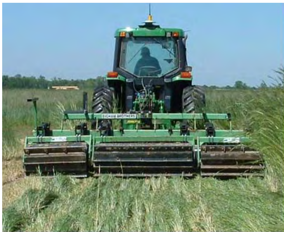
Figure 1. Three-section roller with straight crimping bars 13.5 feet wide.
