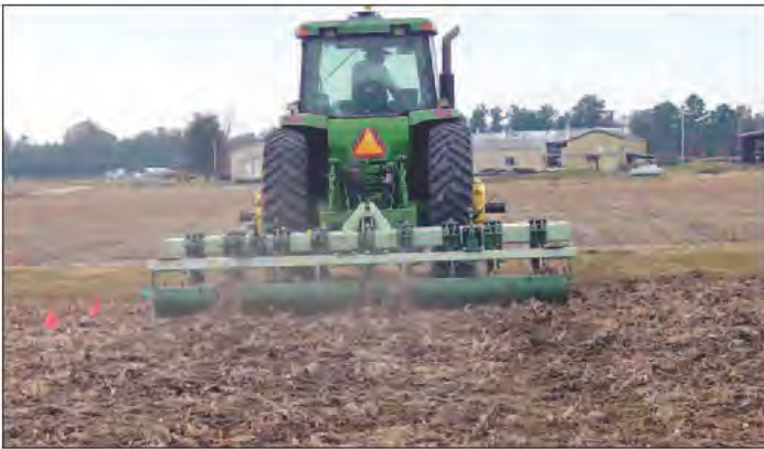
View of subsoiler-leveler operation in the fall.
