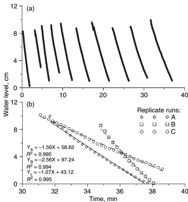
**Figure 2** (a) Representative example of data from an infiltration run with the modified double-ring infiltrometer method. Multiple infiltration events are represented here, until quasi-steady conditions are reached, signalled by the relative small change in slope of the lines (<5%). (b) Example of the final infiltration event for three replicate runs within the same soil using the double-ring infiltrometer method.
