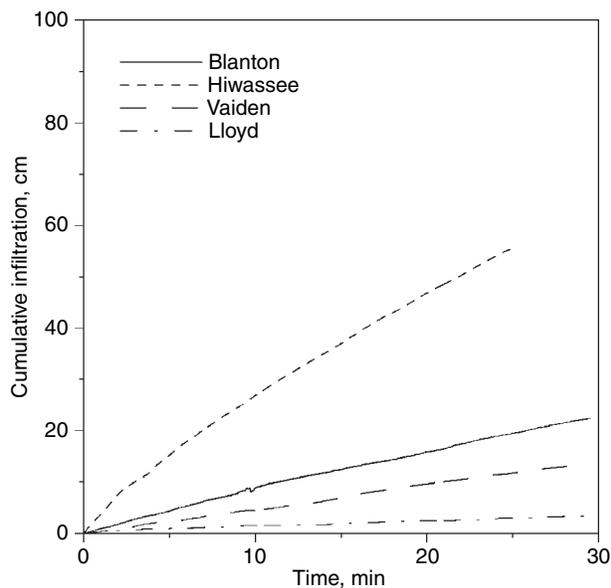
**Figure 3** Cumulative infiltration for the four soil series used to evaluate the automated double-ring infiltrometer method.
