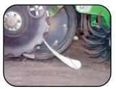
Spoked **closing wheels** offer a good alternative to rubber closing wheels, which can compact the soil surface and cause crusting in heavy, wet soils. Spoked closing wheels, however, can kick out seed with shallow planting.
