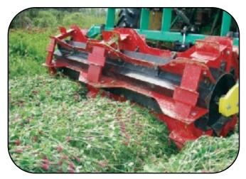
Rotary roller/crimper for elevated bed culture (Kornecki, 2009, U.S. Patent #7,562,517 B1)
