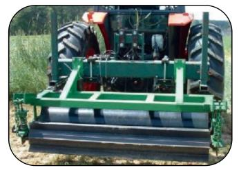
Two-stage roller/crimper (Kornecki, 2011, U.S. Patent #7,987,917 B1)
