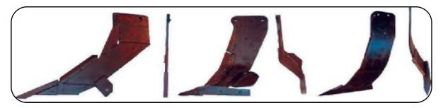
Side and front view of an in-row subsoiler (left) and two bent-leg subsoilders.
