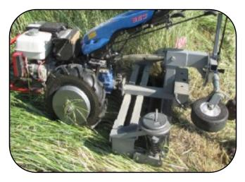
Two-stage roller/crimper for walk-behind tractors (Kornecki, 2011, U.S. Patent #7,987,917 B1)
