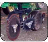
**Double disk openers** create a slot for seed placement. Notched openers can help move residue away from the seedbed to prevent hairpinning.
