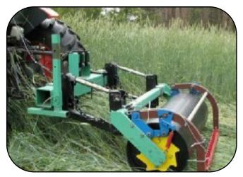
Smooth roller with oscillating crimping bar assembly
