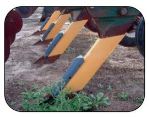
**Polyshields** help prevent soil build-up in heavy or wet soils.
