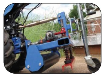
**Powered roller/crimper for walk-behind** (Kornecki, 2012, U.S. Patent #8,176,991 B1)
