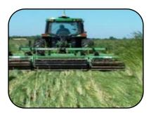
Flattening and crimping cover crops by mechanical rollers is widely used in South America, especially in Brazil, to successfully terminate cover crops without herbicides. Original roller designs consisted of a round drum with blunt,
