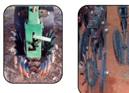
**Down-pressure springs** maintain the desired seeding depth in high residue or on uneven and/or firm ground.
