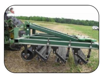
Four-stage roller/crimper (Kornecki, 2011, U.S. Patent #7,987,917 B1)
