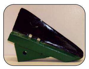
**Splitter points help prevent soil** blowout, especially in dry soils. Newer shanks may incorporate this design, or a piece of metal can be welded perpendicular to the center of a subsoil shank tip.
