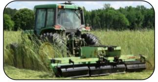
Straight crimping bar roller/crimper
